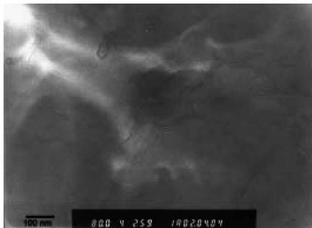
Fig. 13. TEM micrograph of microtomed sample B16 prepared by co-dissolution (Table 2); magnification \times 80k .
