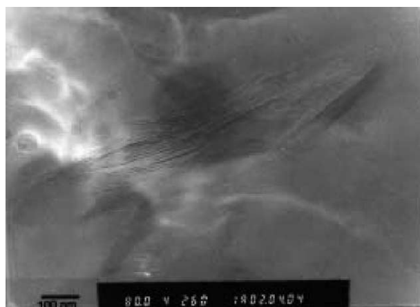
Fig. 12. TEM micrograph of microtomed sample B12 prepared in co-rotating mini-TSE; magnification \times 80k (for SEM see Fig. 8).
